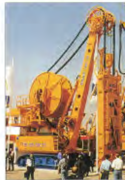
BC 25, cutting depth 30 m
