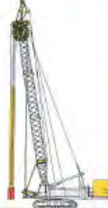
BC 30 on 80 to base machine Height: 29 m Cutting depth: 45 m Operating weight: 26 + 95 t Installed power: 285 + 228 kW
