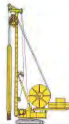
BC 30 with hose drum system on drilling rig BQ 40 Height: 24 m Cutting depth: 60 m Operating weight: 35 + 115 t Installed power: 300 + 400 kW
