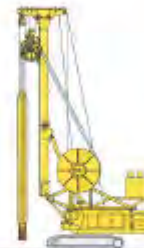
BC 30 with cutter base system and hose drum system on 120 to base machine Height: 24 m Cutting depth: 30 m Operating weight: 35 + 100 t Installed power: 500 kW
