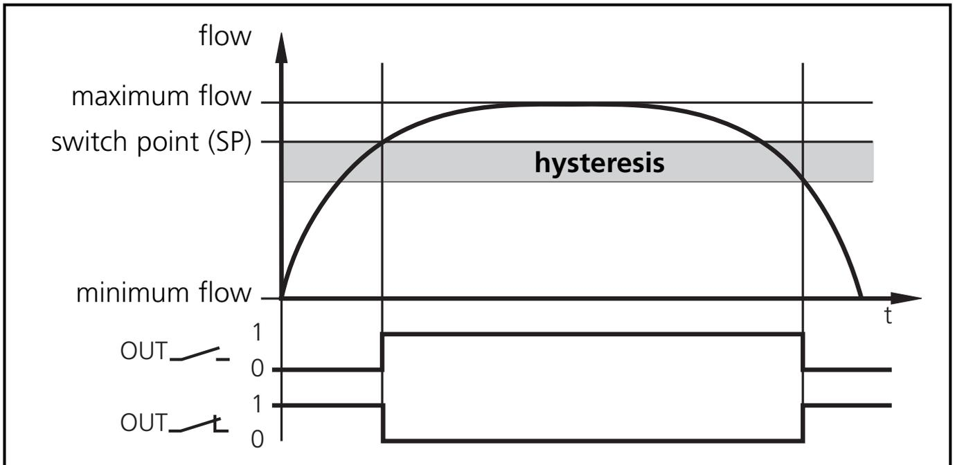
When the flow rises, the output switches when the switch point (SP) has been reached.
