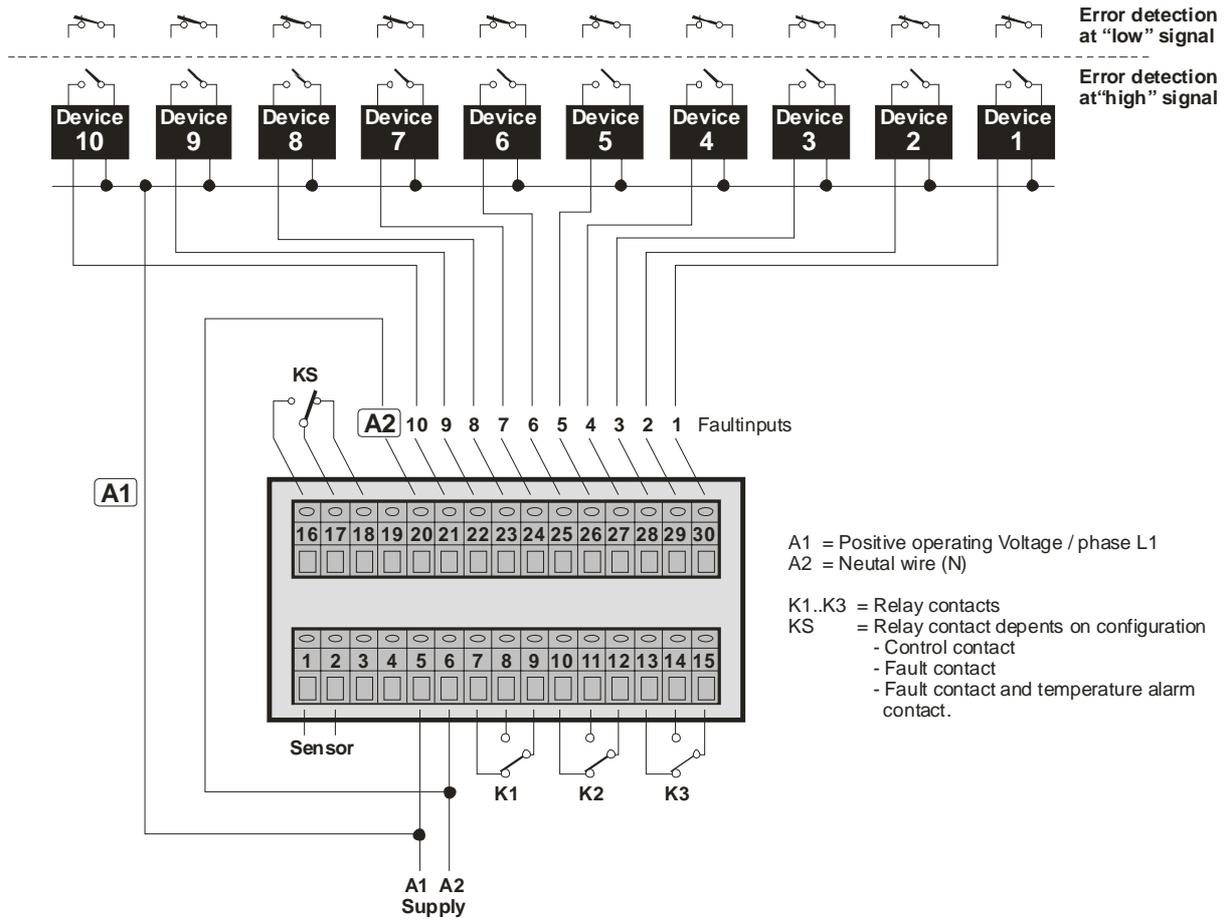
**Connecting diagram** (the right number of replays are shown of the device label)
