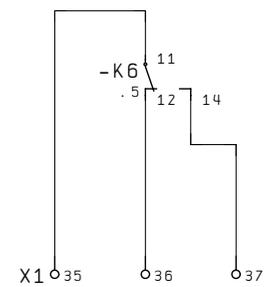
Fault signal contact
