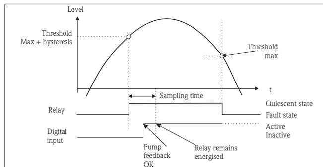
Fig. 14: Pump monitoring, pump OK
