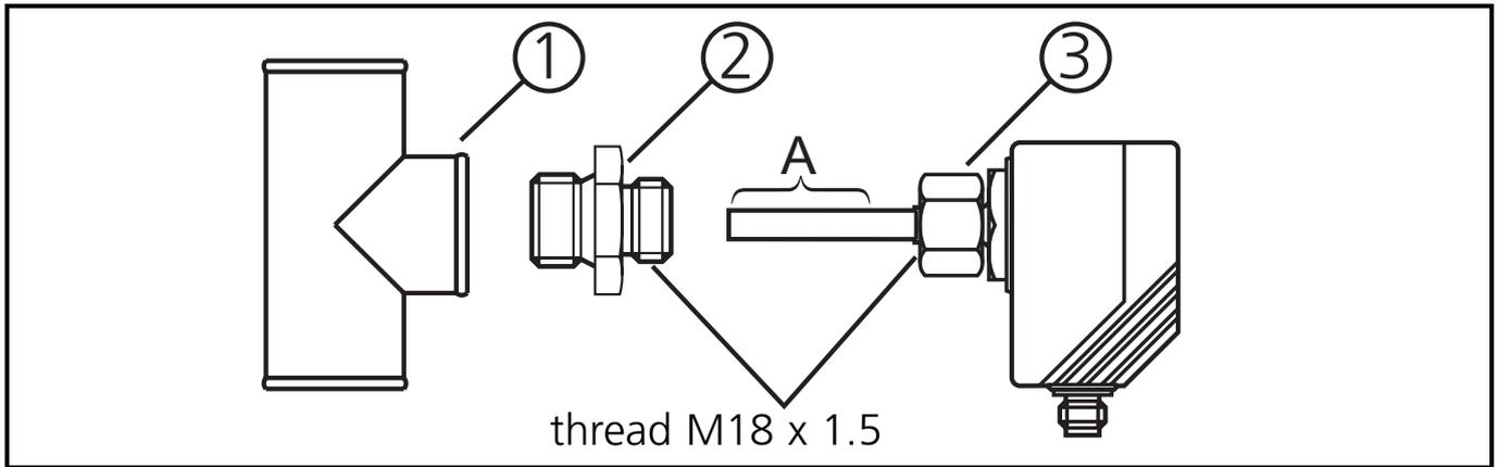
1. Lubricate the nut (3) and all threads with grease to ensure the nut can be loosened and tightened several times.
