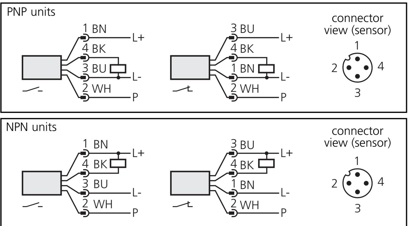
P = programming wire (for remote adjustment)
