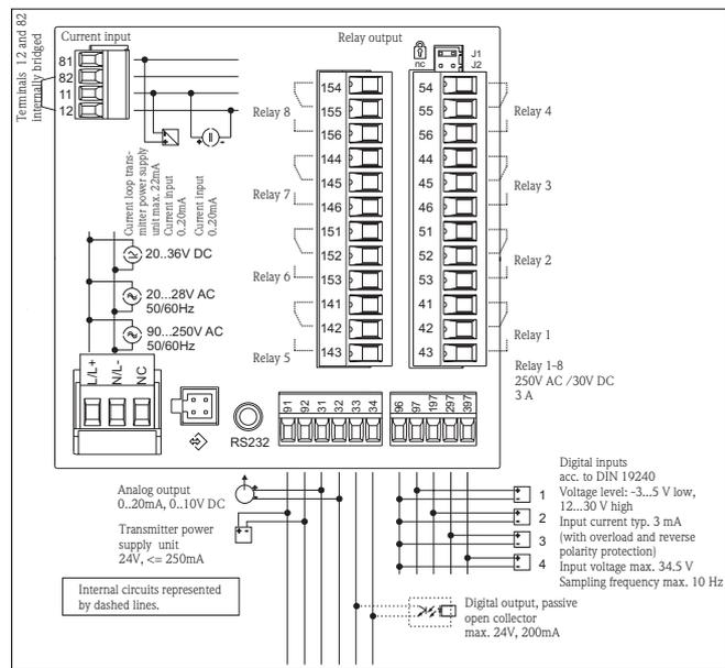
Fig. 22: Terminal assignment of process display unit
