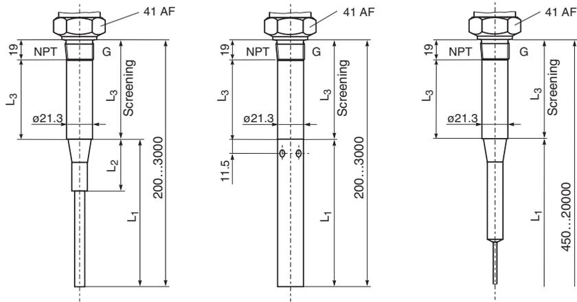
Probes with **active build-up compensation** (always 100 mm)
