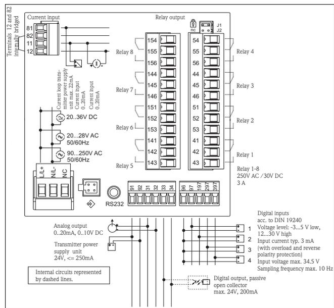
Fig. 4: Terminal assignment of process display unit (Universal input see Page 58)
