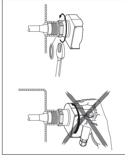
Probe with parallel thread G 3/4 A and with sealing ring: Tighten at the hexagonal nut to max. 100 Nm (G 1 A to max. 180 Nm)
