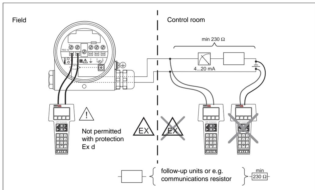
A load should be connected into the power cable when connecting a handheld terminal. The handheld terminal can now be connected at any point along the power cable for communication with the electronic insert. The size of the load is given in the following table.
