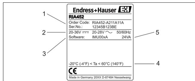
Fig. 2: Nameplate of the process display unit (example)
