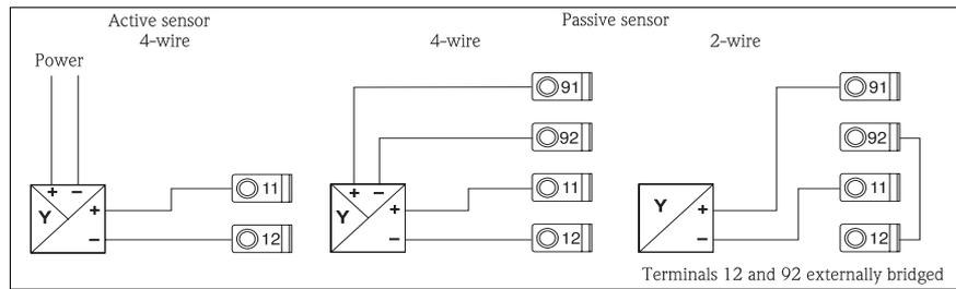
Fig. 8: Connecting a sensor to universal input
