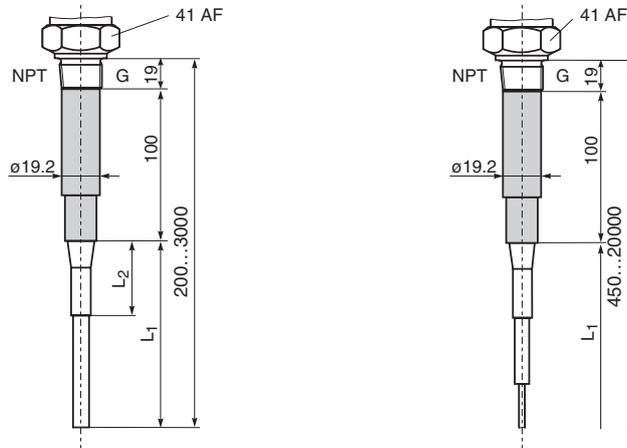
Probes with **screening L3** and with **active build-up compensation**
