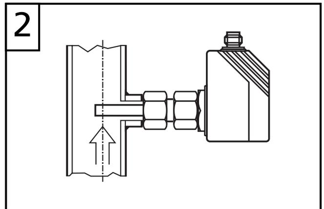
To avoid malfunction a minimum distance between the flow monitor and bends, valves, changes in cross-section or such like must be observed:
