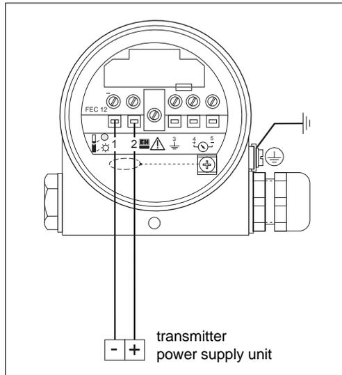
Insert the power cable through the cable entry on the probe housing. Unscreened or general purpose multi-core cable can be used as the connecting cable. If strong electromagnetic interference occurs due to, e.g. machinery or radios, then screened cable, grounded at the probe end, should be used. Connect the screening to the ground terminal on the probe housing.
